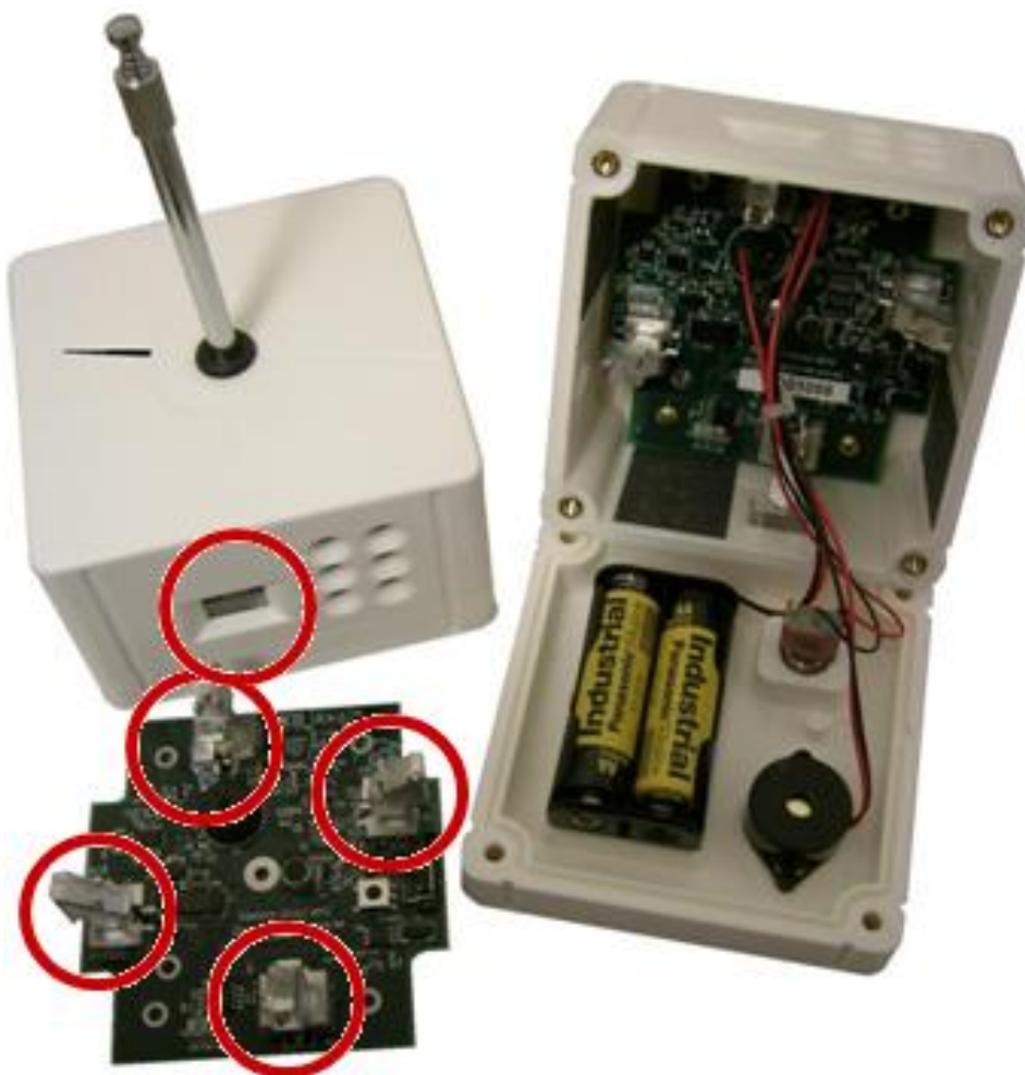
Figure 6.2: XSM circuit board with integrated PIR sensors and the XSM ruggedized enclosure. The red circles show the PIR sensors on the board as well as on the enclosure (Figure courtesy EECS, UC Berkeley and CrossBow Technology)
